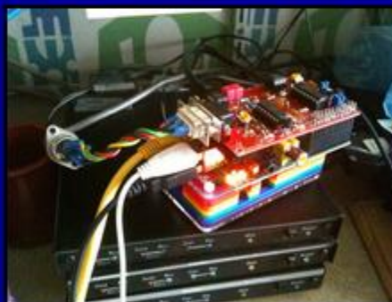
Raspberry Pi - TNC-Pi - AX.25 1200 bauds
